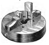
some of these chucks the jaws are operated simultaneously by a right and left-hand screw, while in others, each jaw has its own separate screw.
