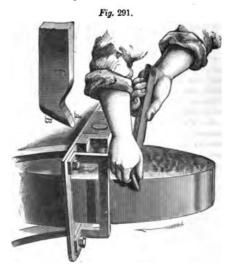
instant too long in either of the positions indicated by the dotted lines, G, H, or at any time during the motion, a hollow spot will be ground upon the tool at the point of contact between the stone and the tool; furthermore the grinding operation is not very accessible to the eye and hence any irregularities are not very easily corrected.
